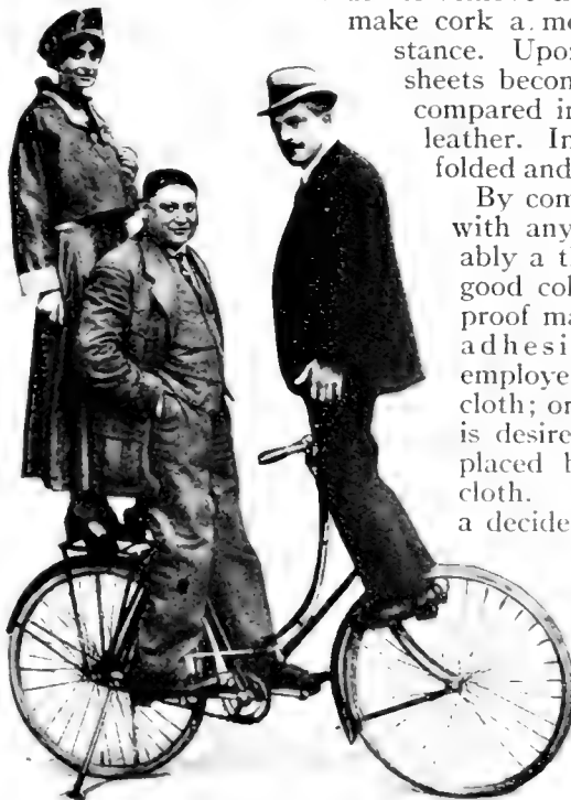
The steel rod supports are strong enough to sustain a combined weight of eight hundred pounds
